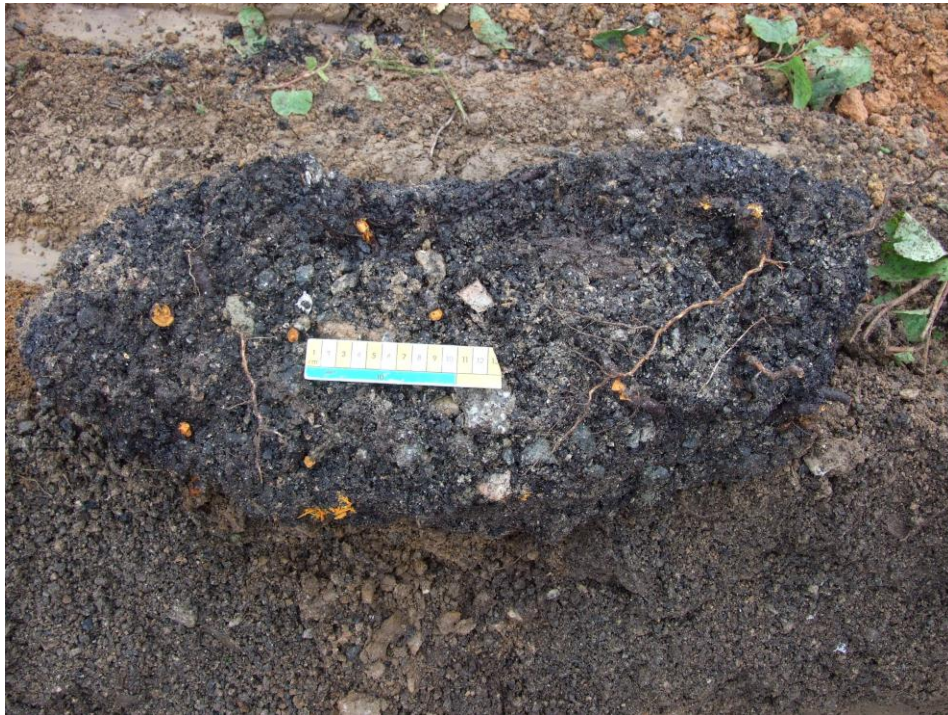
Fig.4.34 Rhizome penetrating tarmacadam
