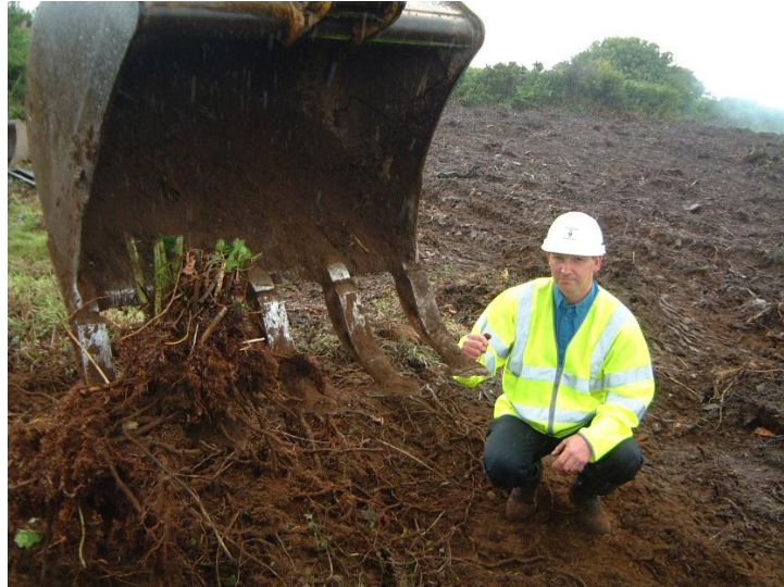
Fig. 4.5 Extended tines on excavation machinery
