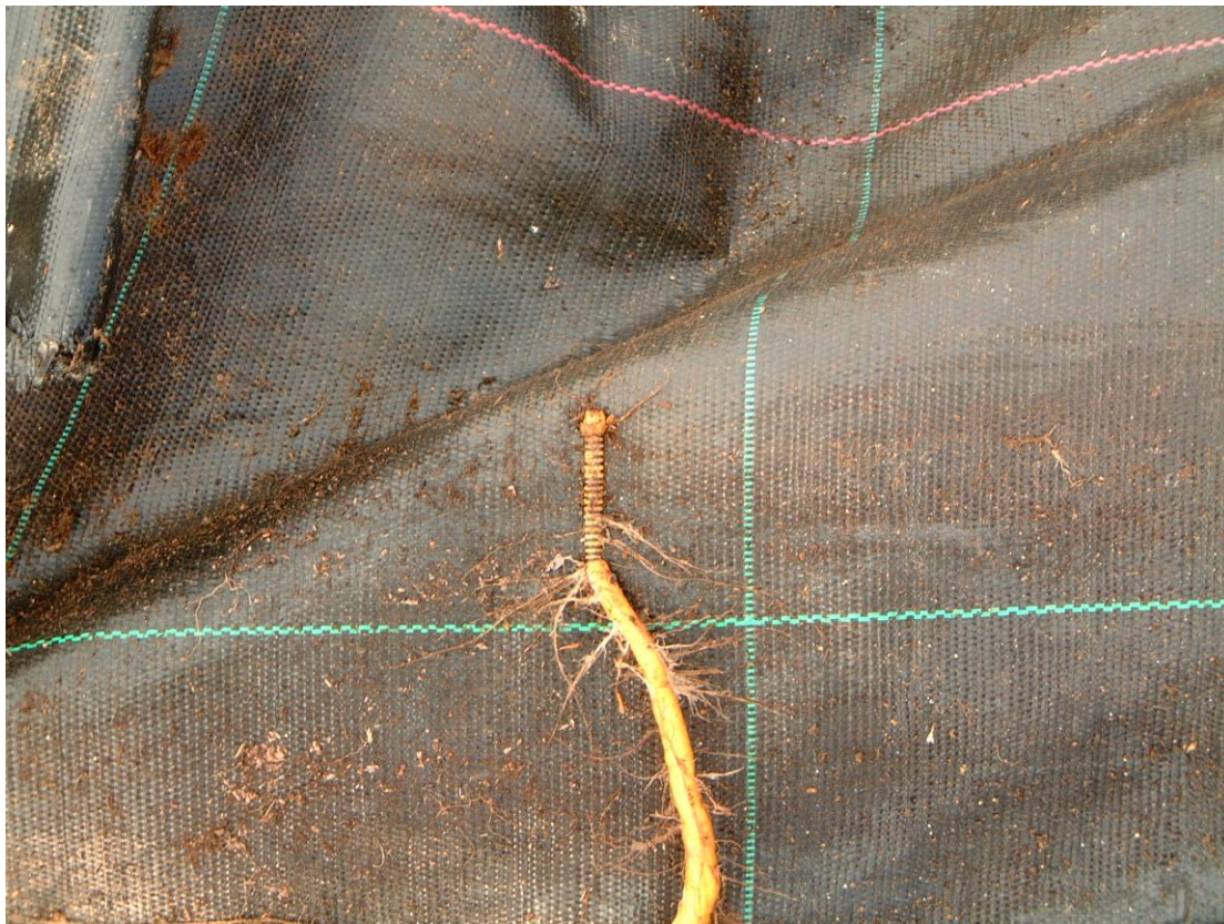
Fig. 3.41 Detail of underside of barrier material showing root and detail of constraint
