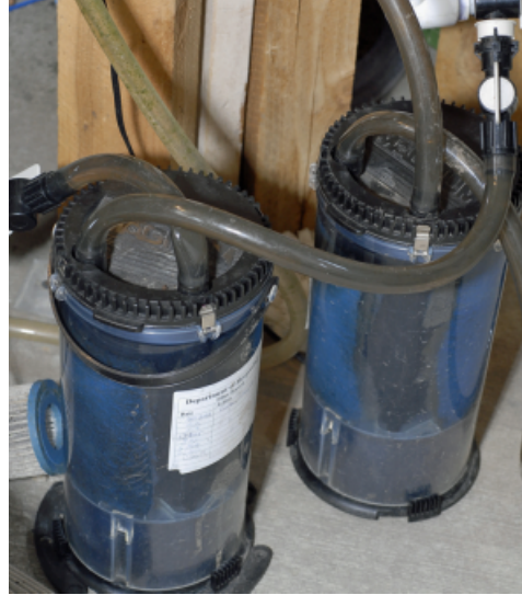
Plate 1. A common design for a canister filter. Depending on the media installed, these filters can provide mechanical, chemical and even biological filtration. R. A. Odum, Toledo Zoological Society.
