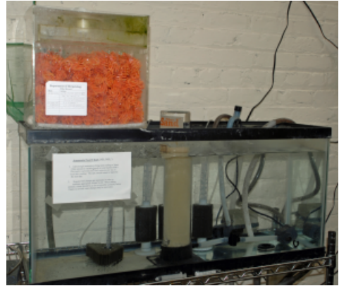
Plate 3. A biofilter cycling tank. Different types of biofilters, including trickle, sponge and fluidized bed filters, are cycled in this tank using an artificial source of wastes (ammonia). These filters can then be transferred to other tanks containing animals, without cause for concern about transferring pathogens between groups. Note the instructions to the keeper for daily maintenance on the left side of the tank. R. A. Odum, Toledo Zoological Society.
